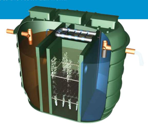
The FlowPath contains two stage primary settlement zones, designed to settle coarse and non-biological loadings.
