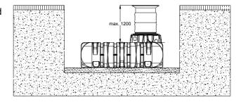
Cover heights with cast iron telescopic dome shaft (class B) in area driven over by vehicles up to 3.5 tonnes.
