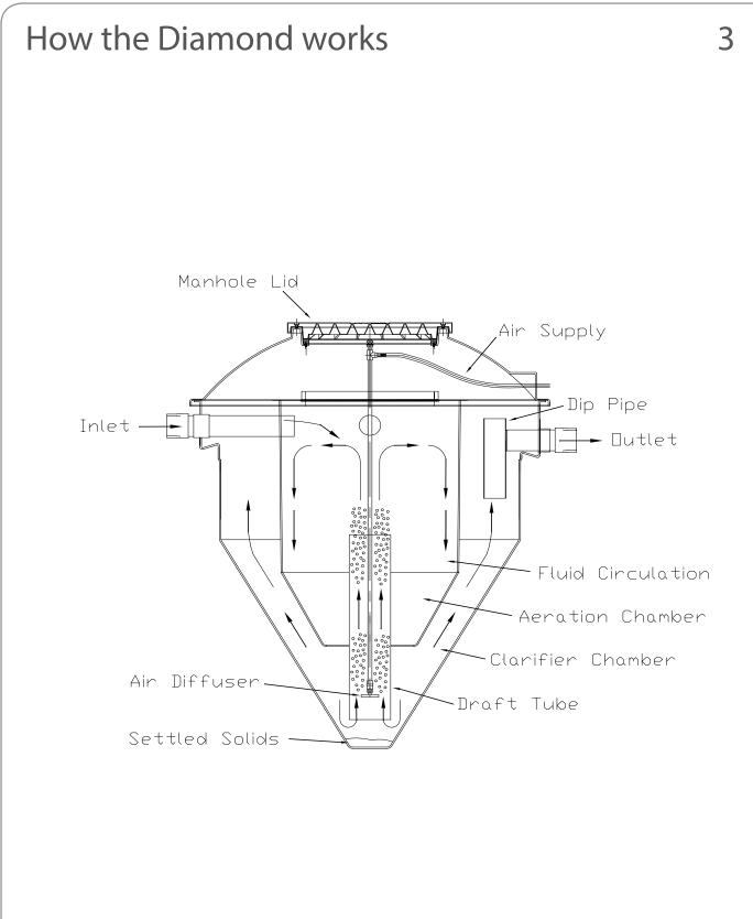
The sectional drawing above shows a typical DMS treatment tank but the larger DMC models work on exactly the same principle. To calculate the trench size for the Diamond plant to be installed refer to the size chart and groundworks diagram on page 6 & 9.
