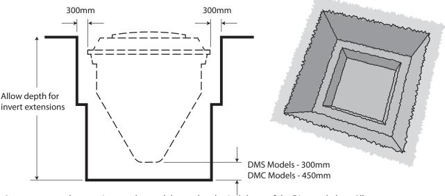
A square stepped excavation may be used due to the physical shape of the Diamond plant. Allow adequate clearance for all pipes and any other connections the unit.
